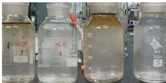
▶ Comparison of Influent and Effluent of Tank Farm Oil Wastewater Treatment Project of a Refining-Petrochemical Enterprise
