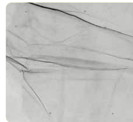
► Graphene Oxide TEM
