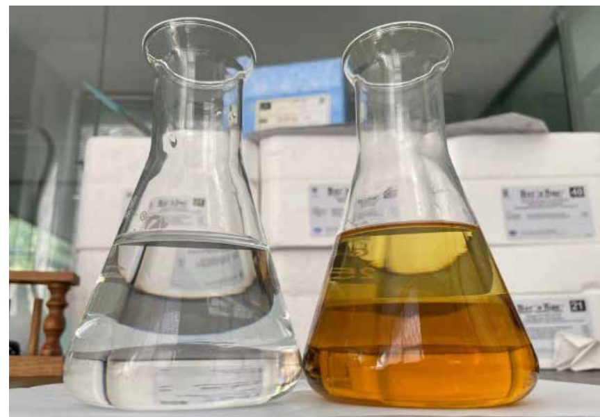
► Contrast Before and After Absorption of Amine Solution
