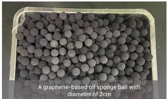
A graphene-based oil sponge ball with a diameter of 6cm
