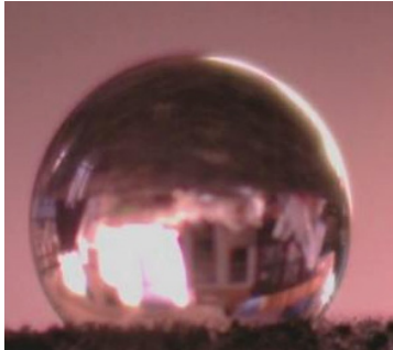
Graphene-based oil sponge water contact angle test diagram
