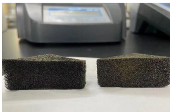
○ Pictured above is a new graphene-based oil sponge with a graphene-based oil sponge that has been reused more than 1,000 times
