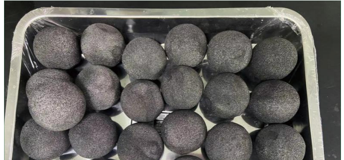
A graphene-based oil sponge ball with a diameter of 6cm
