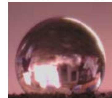
Graphene-based oil sponge water contact angle test diagram
