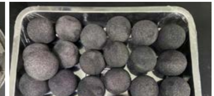
A graphene-based oil sponge ball with a diameter of 6cm
