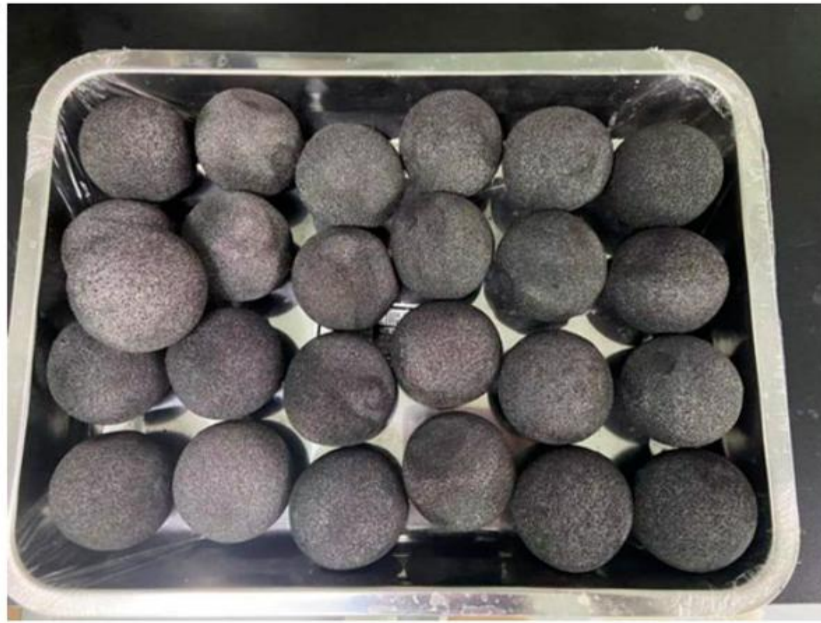
Graphene modified sponge ball with 6cm diameter
