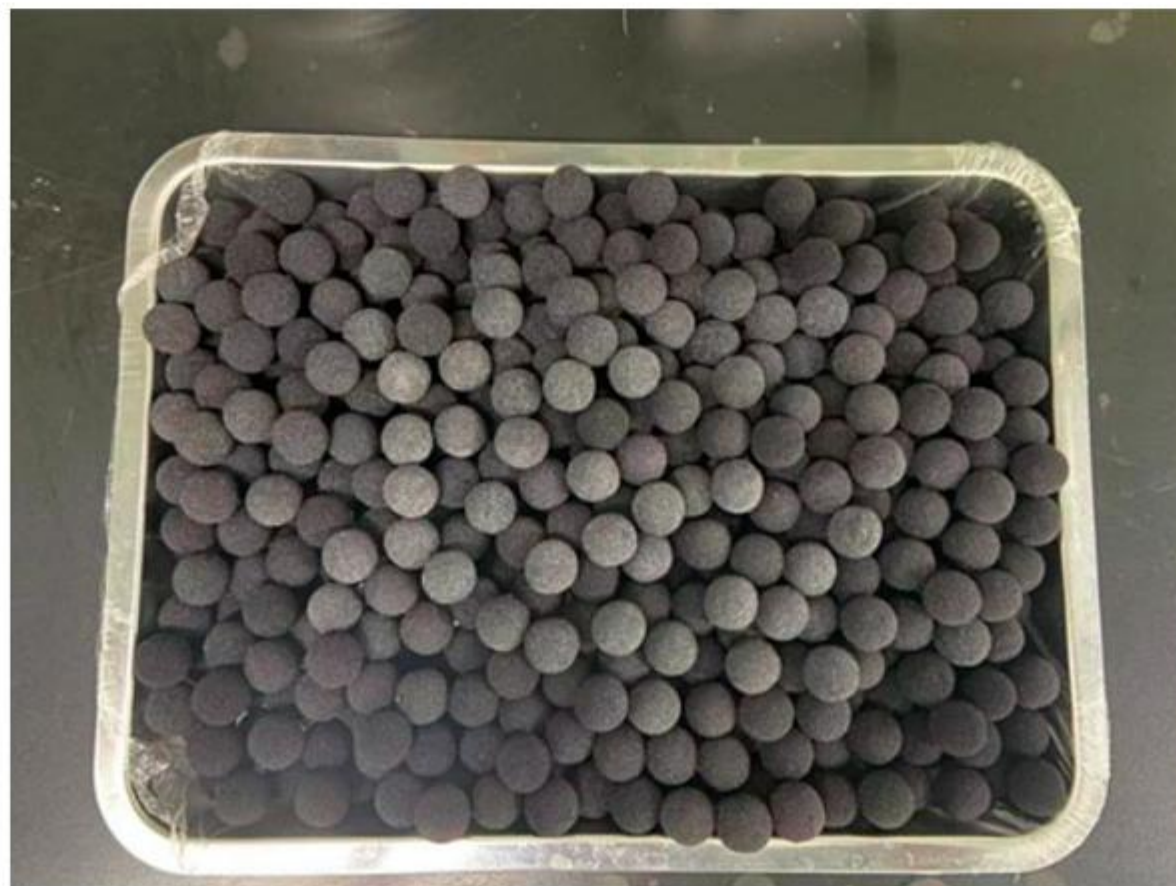
Graphene based oil sponge ball with 2cm diameter
