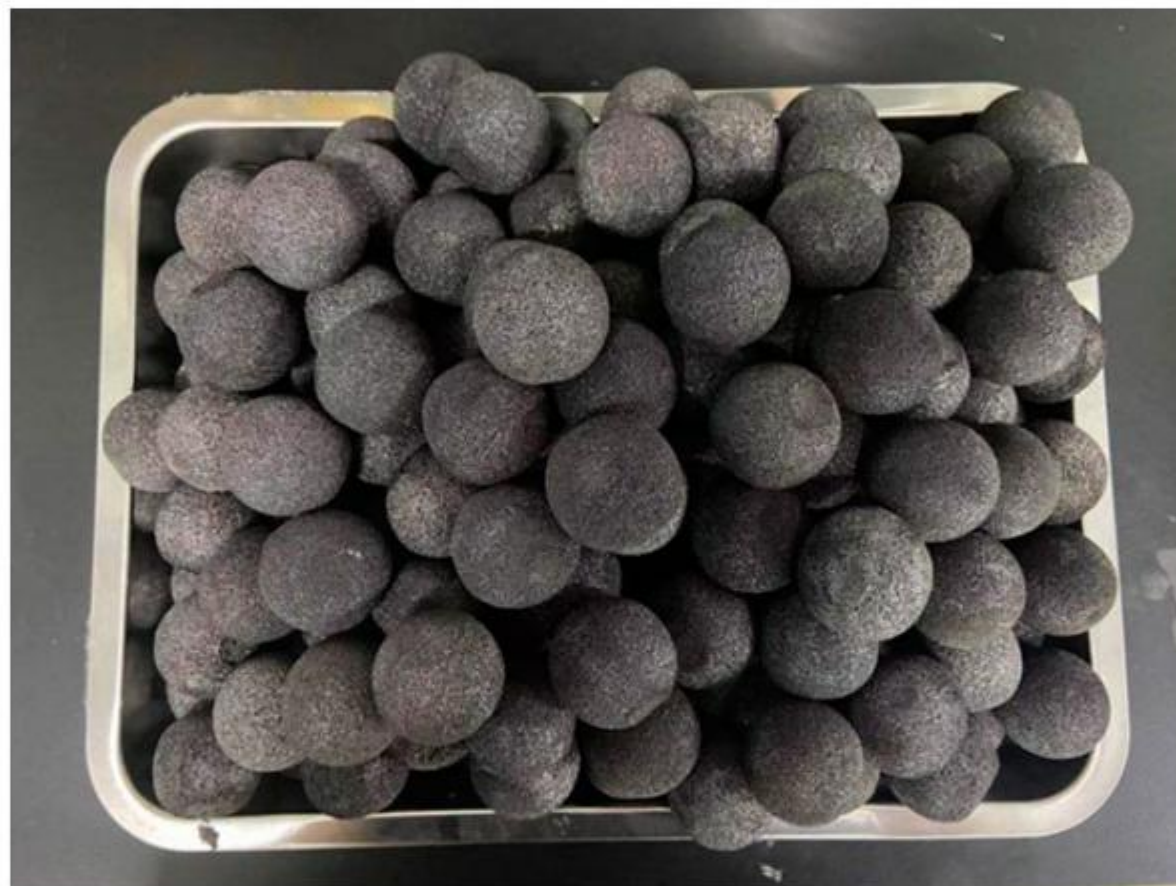
Graphene based oil sponge ball with 4cm diameter
