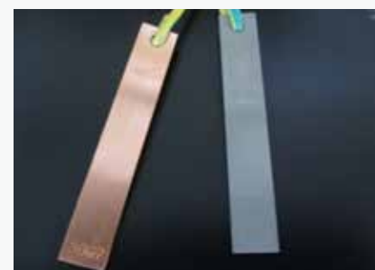
► Before adding the corrosion and scale inhibitor
