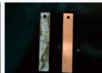
► Add corrosion inhibitor corrosion effect
