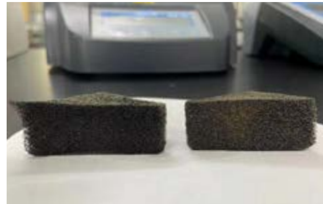
○ Pictured above is a new graphene-based oil sponge with a graphene-based oil sponge that has been reused more than 1,000 times
